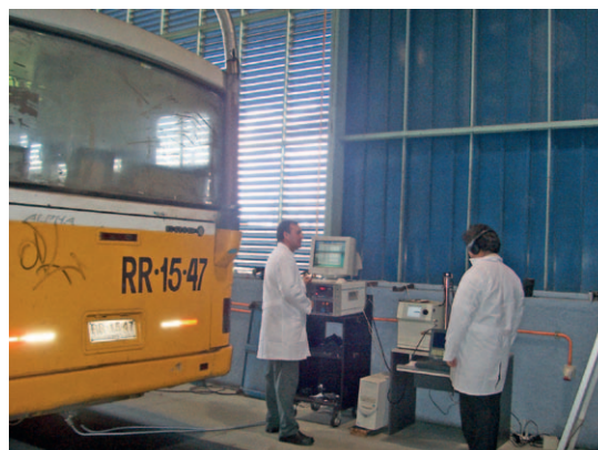
Measurements with NanoMet during pilot program (2004). Source: 3CV.
