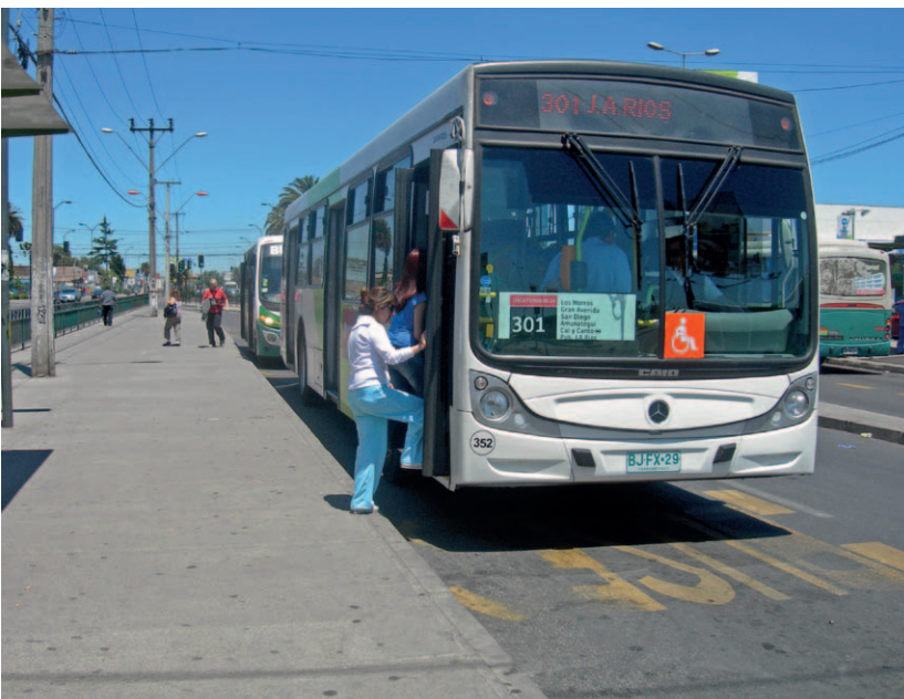
DPF equipped bus, acquired after coming into force of the modification of Supreme Decree N° 130.
