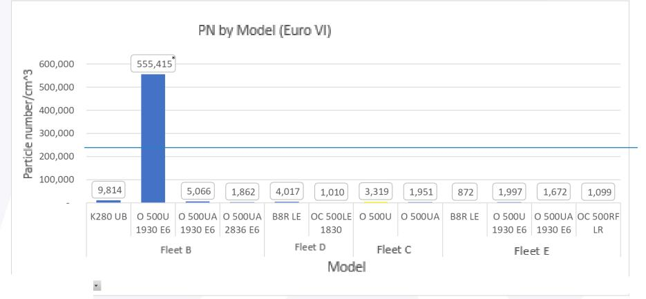
A single O-500U 1930 marked over 10.000.000 PN/cm^3. This value is associated to poor maintenance and increased average 99+% of new Euro VI buses approve pass/fail criteria
