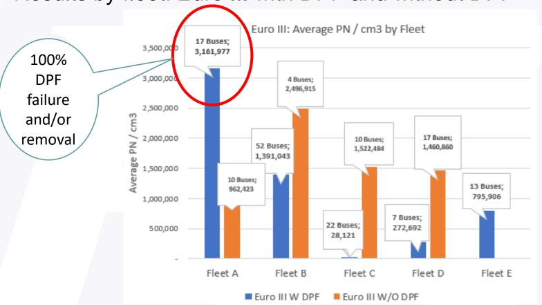
DPFs reduce significantly the particle numbers but maintenance is required to ensure optimal performance. The fleets with best maintenance have the lowest emissions
