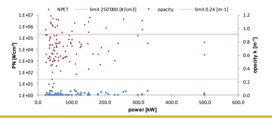
Failures do not depend on engine power, operation time, immatriculation year nor brand These failures are random, missing maintenance or manipulation - only detectable by 100% PTI
