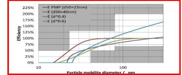
Figure 2: Schema of the limits for the number concentration efficiency curve (white area) and examples of efficiency curves conform to the requirements (curves)
